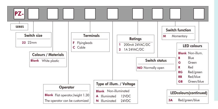
Plastic piezo switches offering rugged, sealed tamper and vandal proof solid state switching. Exceptional durability and reliability. Fitted with red, green and blue LED's for illumination.
